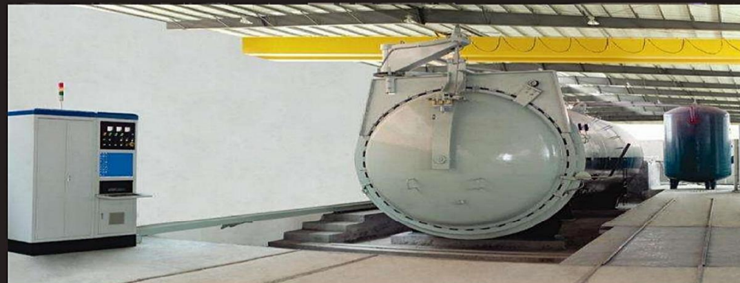
夹胶生产线大型高压釜设备 Laminated production line of large autoclave equipment
