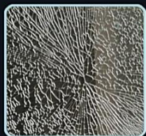
钢化玻璃破碎后成细小颗粒状 Tempered glass after breaking into a small granular
