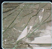
普通玻璃破碎后成尖锐刀状 Ordinary glass broken into a sharp knife
