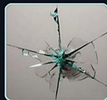
半钢化玻璃破碎状 Semi tempered glass broken
